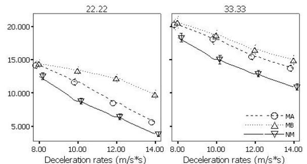
Figure 5. Minimum following distance after LV's braking (m)
