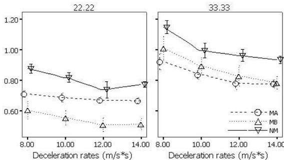
Figure 3. Time of first pressing brake pedal (in seconds)
