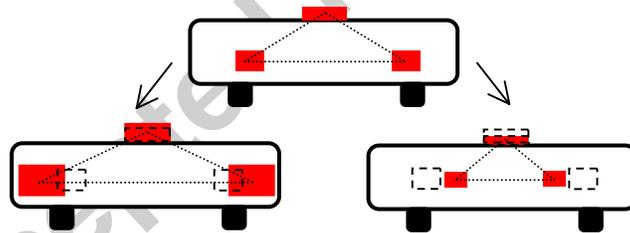
Figure 2. Rear view sketch of LV, showing manipulation of separation and size of the brake lights during LV braking. Top represents normal pattern of brake lights. Bottom left illustrates expanded brake lights and bottom right represents contracted brake lights. Normal (top) pattern is shown for comparison as dashed lines. Note that only initial and final stages are shown here; the actual manipulation involves a *continuous* process during braking.
