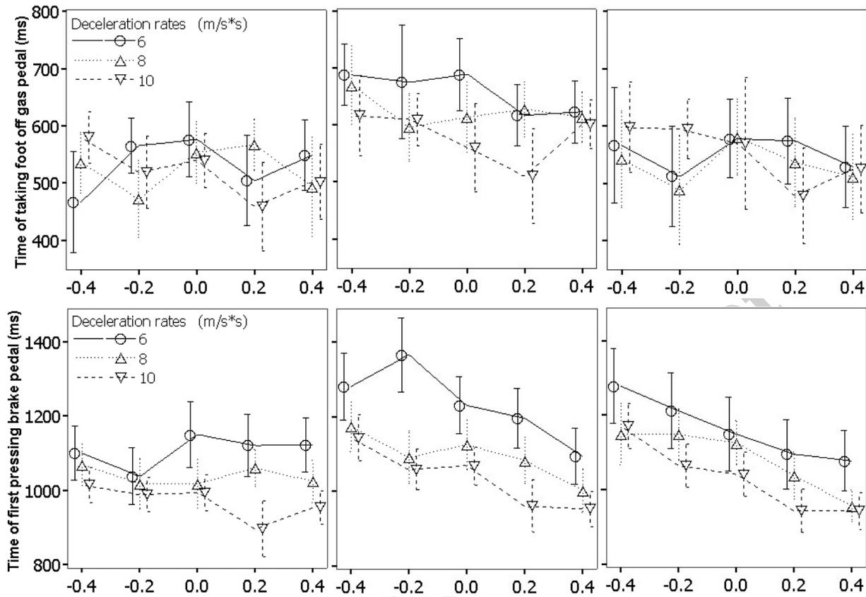
Figure 5. Top: Time of taking foot off gas pedal; bottom: time of first pressing brake pedal (both in ms). In all graphs, data are averaged across 3 viewing conditions and 3 deceleration rates, under 5 manipulation conditions. Error bars represent 95% confidence intervals. Positive, zero and negative times represent after, at, and before the start of LV braking.
