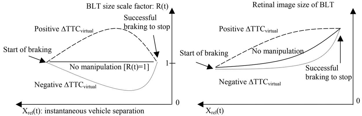
Figure 4. Qualitative illustration of changes of scale factor and retinal image size versus vehicle separation during LV braking. Left: BLT size manipulation based on  $\Delta\text{TTC}_{\text{virtual}}$ ; right: retinal expansion of BLT on eye of the FD while LV is braking. Solid lines represent no manipulation; dashed lines represent expansion; dotted lines represent contraction. Note:  $R(t)=1$  represents original, normal size of LV.
