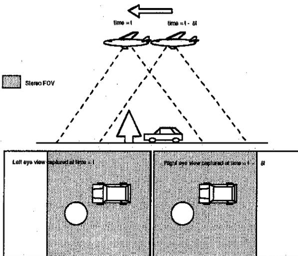
Figure 1 - Stereo pair created using the single camera, hyper-stereoscopic video system.
